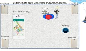
The GEPPS™ system consists of an infrastructure that collects information from the positioning tag. How far tag is located from a certain Sense point is measured and send to the cloud server. The server calculates each tags position to APP or Monitor
