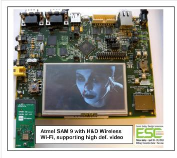
Photo: Atmel SAM9M10 capable to handle multimedia playback and streaming using Bonjour<sup>™</sup> service discovery over the Wi-Fi connection provided by H&D Wireless AB.
